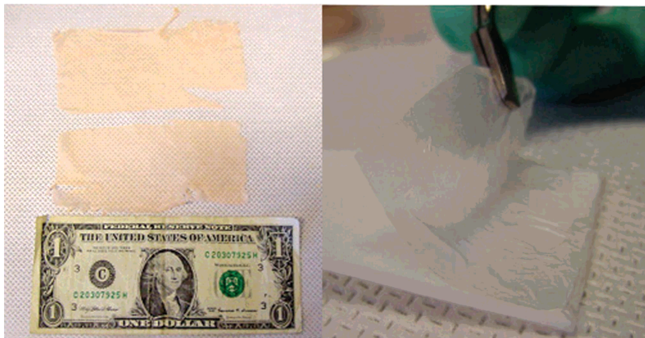
Figure 2. Isolated layer-by-layer PEO/PAA assembled at pH 2.5. Both films shown, isolated from a Teflon substrate, were clear and flexible.
